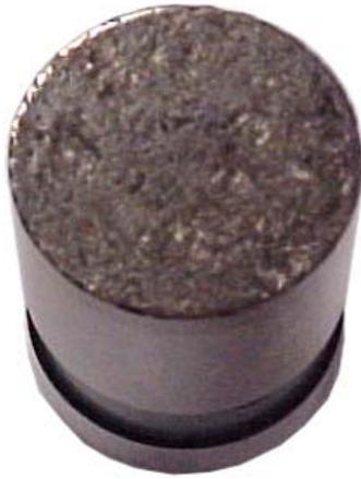
**FIGURE 9 REPLACEMENT SIGNATURES, SPALLED LIFTER**
