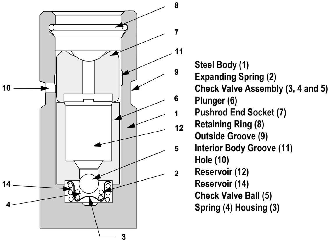
**FIGURE 2 HYDRAULIC LIFTER CROSS SECTION**
