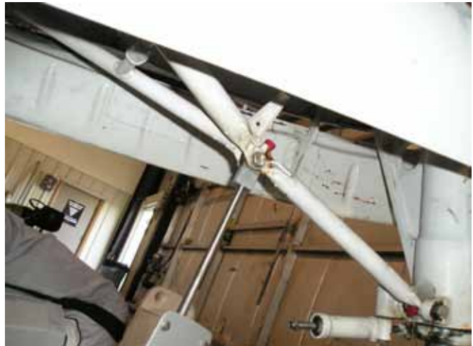
Checking the nose gear down tension with a mechanical push-pull force gauge.
