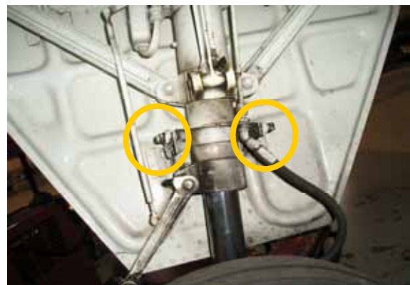
Outer gear door connection points
