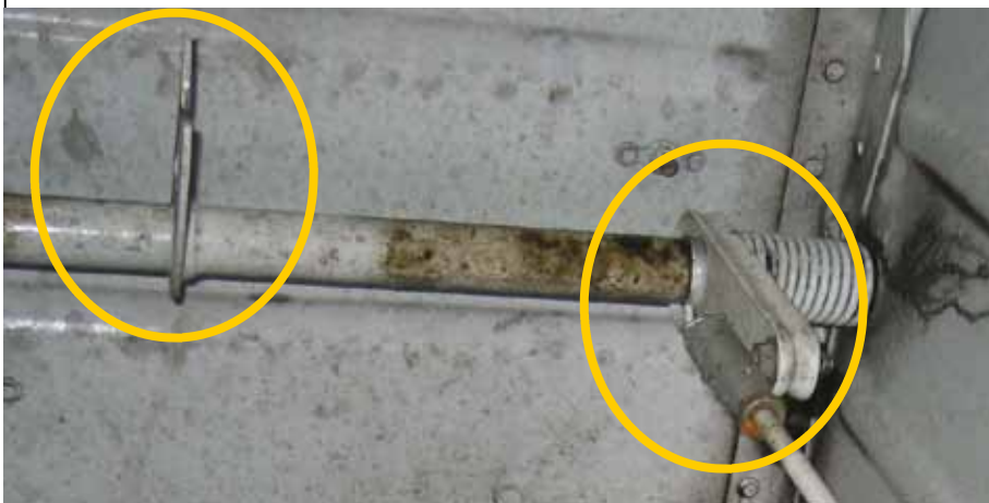
Nose gear door actuator arm (right) and door actuator pin guide (left)
