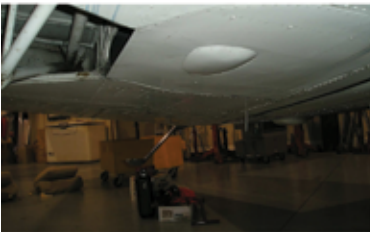
Main gear inner door in fully retracted position
