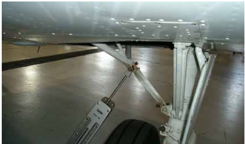
Checking the nose gear down tension with a mechanical push-pull force gauge.
