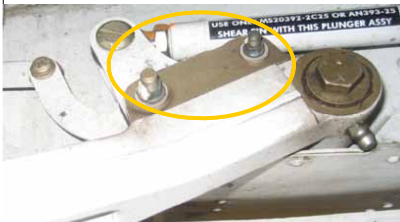
Retract rod mounting bolts
