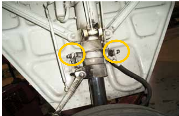
Outer gear door disconnect points
