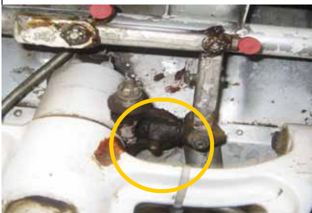
(above) Properly installed grease zerk, pointed down.
